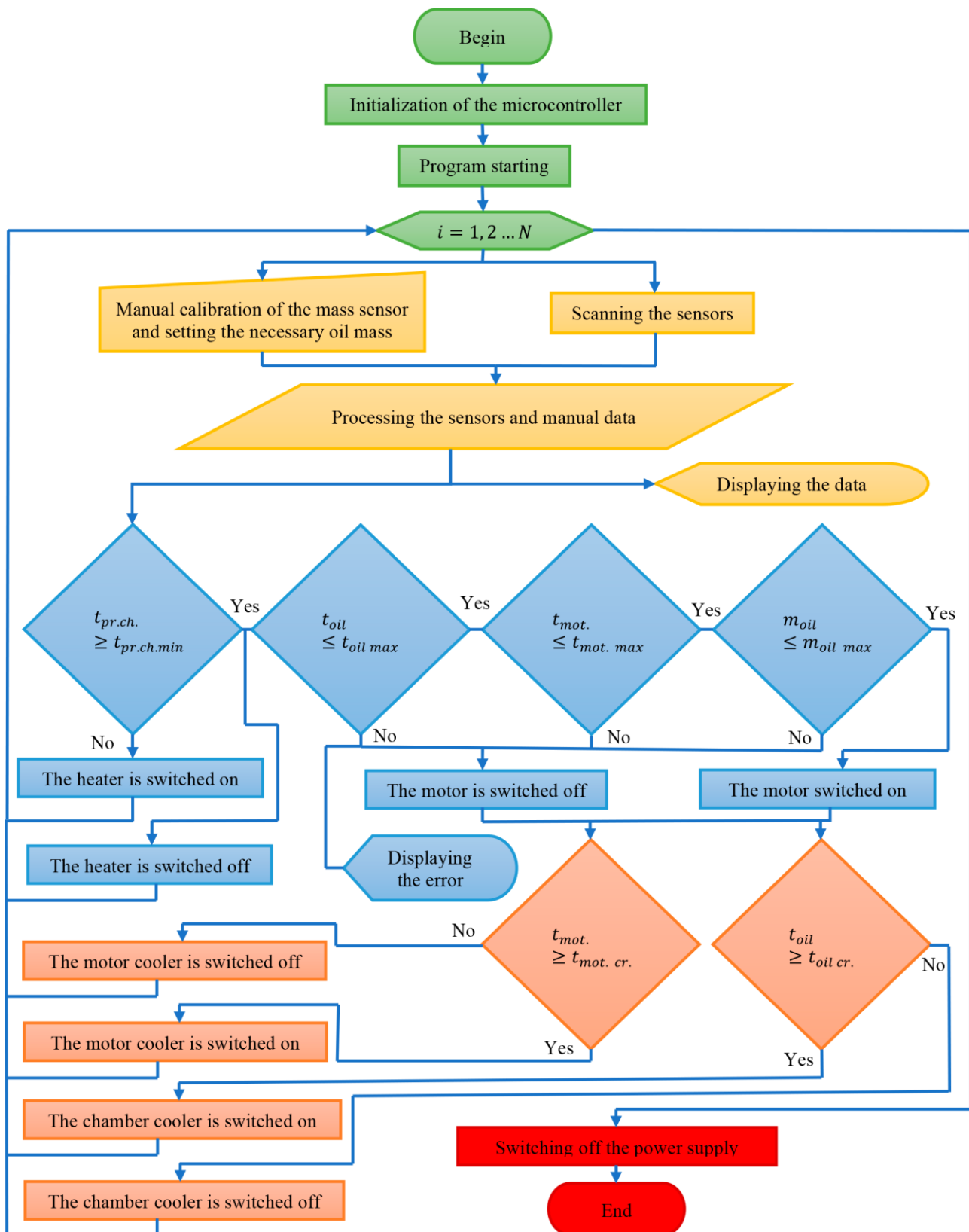
Fig. 3. Simplified block diagram (flow chart) describing the general algorithm of the control system operation
