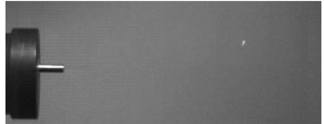
Fig. 2. The sample at the moment it hits the anvil
