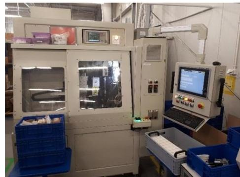
Fig. 4. Test stand for testing hydraulic solenoid valves
