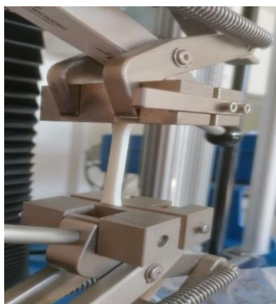
Fig. 4. Appearance of samples during stress relaxation tests
