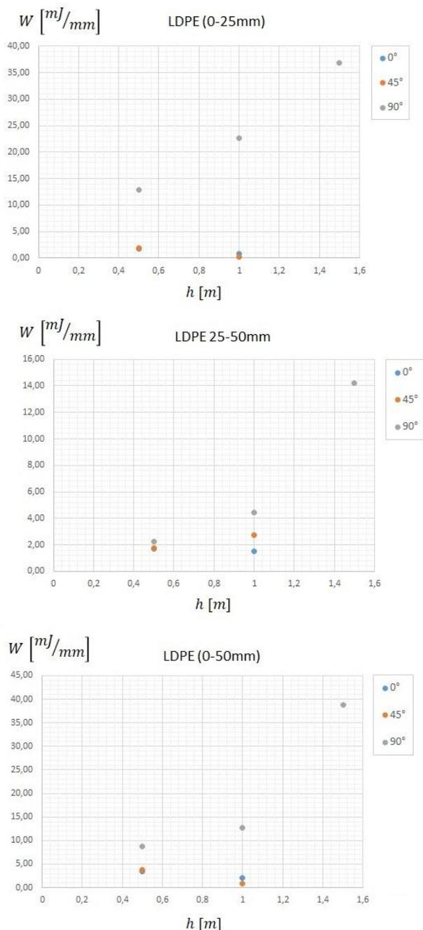
**Fig. 15.** Work of deformation per unit length  $W$  [ $mJ/mm$ ] as a function of flail drop heights  $h$  [ $m$ ] calculated for  $\varepsilon = 0.15$ . Results for angles:  $0^\circ$ ,  $45^\circ$  and  $90^\circ$  and three measuring sections 0-25mm, 25-50mm and 0-50mm
