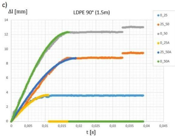
Fig. 12. Dynamic elongation  $\Delta l$  [mm] as a function of time for angles: 0°, 45° and 90° and 1.5m drop height
