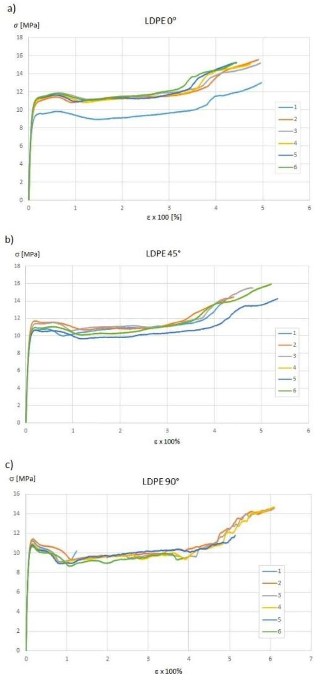
Fig. 3. Static stress  $\sigma$  on relative strain  $\epsilon$  for angles: 0°, 45° and 90°
