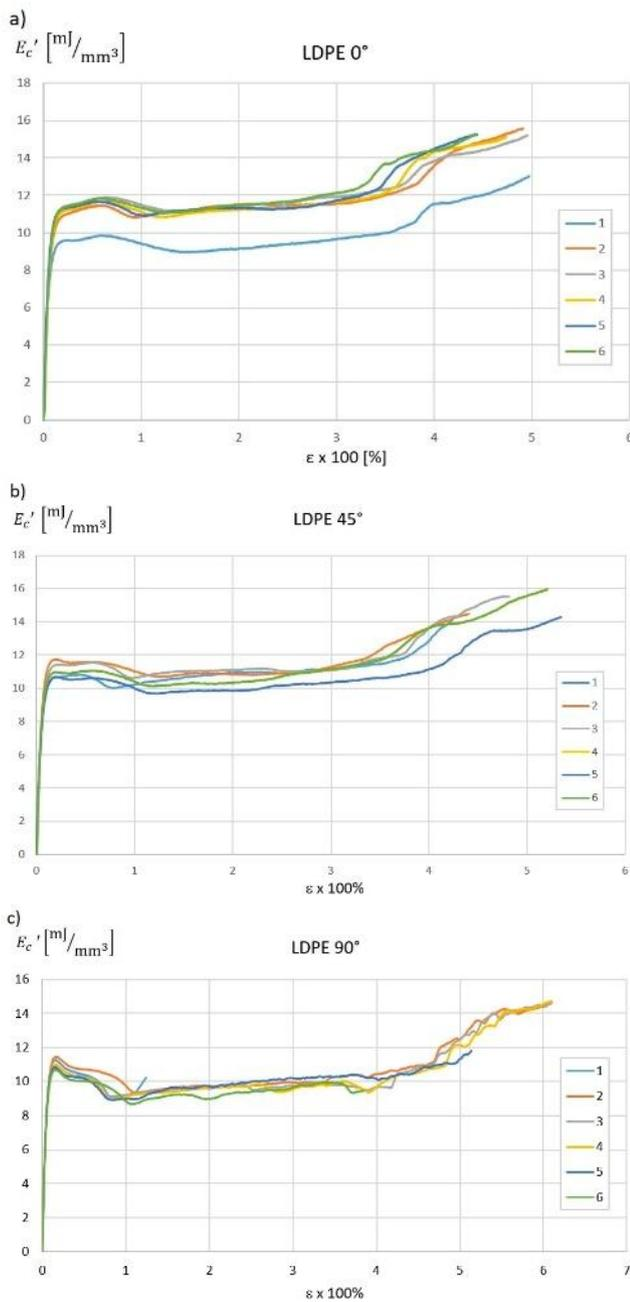
Fig. 6. Volumetric Energy change intensity  $E_c'$  [ $mJ/mm^3$ ] on relative strain  $\varepsilon$  for angles:  $0^\circ$ ,  $45^\circ$  and  $90^\circ$
