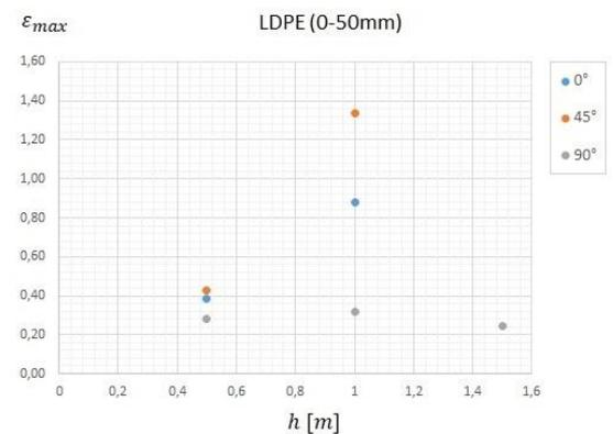
Fig. 14. Relative strain  $\epsilon$  as a function of flail drop heights  $h$  [m]. Results for angles: 0°, 45° and 90° and three measuring sections 0-25mm, 25-50mm and 0-50mm
