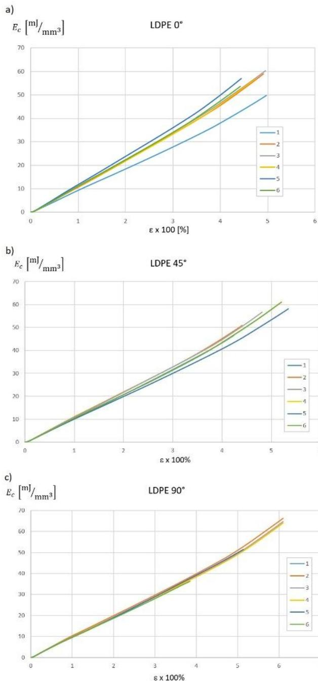
Fig. 5. Static energy density  $E_c$  [mJ/mm<sup>3</sup>] on relative strain  $\epsilon$  for angles: 0°, 45° and 90°
